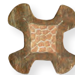
Indenter Crimp Cross-Section Across Axis
